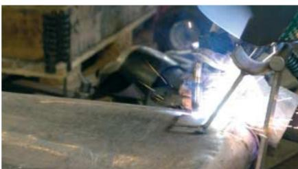
Welding of a stainless bearing construction element for the process industry. Quattro Pulse is often used for sheet metals down to 1 mm to ensure a minimum of heat input.
