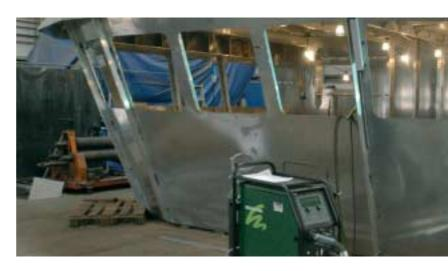
Construction of large aluminium tanks in hardening material. The welding machine is configured with watercooling and Push Pull torch for up to 1.2 mm wire diameter.
