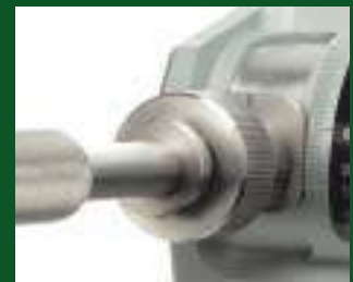
Eccentric plate triples the use of the diamond wheel.
